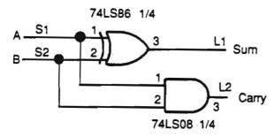
FIGURE 6-15. Half-Adder Schematic.
