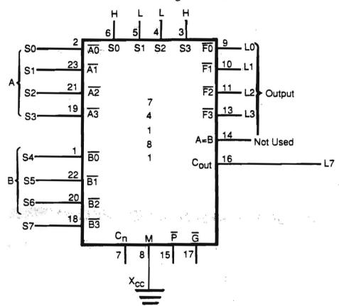
3. Place all logic switches to off. Turn on power. D1 and L7 should light. Use S0-S3 as the A input, S4-S7 as the B input, L0-L3 as the F output and L7 as the carry output. Observe and describe the action of this circuit. Remember that the carry output is LO true.
